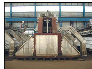
Finished POT Assembly for BALCO at Korba
